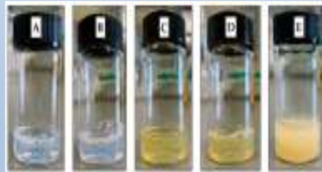
Figure 7. Visual appearance of the nanomicelles. (A) Empty polymeric nanomicelles (PNM); (B) Empty mixed nanomicelles (MNM); (C) Silymarin (SLM)-loaded PNM; (D) SLM-loaded MNM; (E) SLM aqueous suspension.
